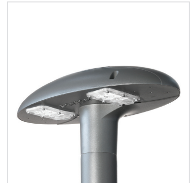
The ProFlex™ optical units are turned 90° for asymmetrical light distributions.
