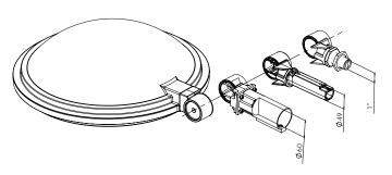
MOUNTING WITH KNUCKLE JOINT Female, on a plain spigot (D60F) Male, on a female spigot (R/D6oM) Male, on a 1" BSP threaded tube (R/G34M)
